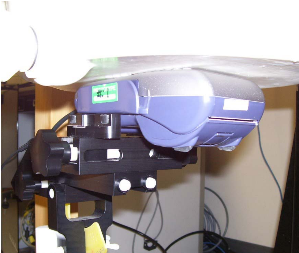
Front Side of EUT against Phantom with External Power
