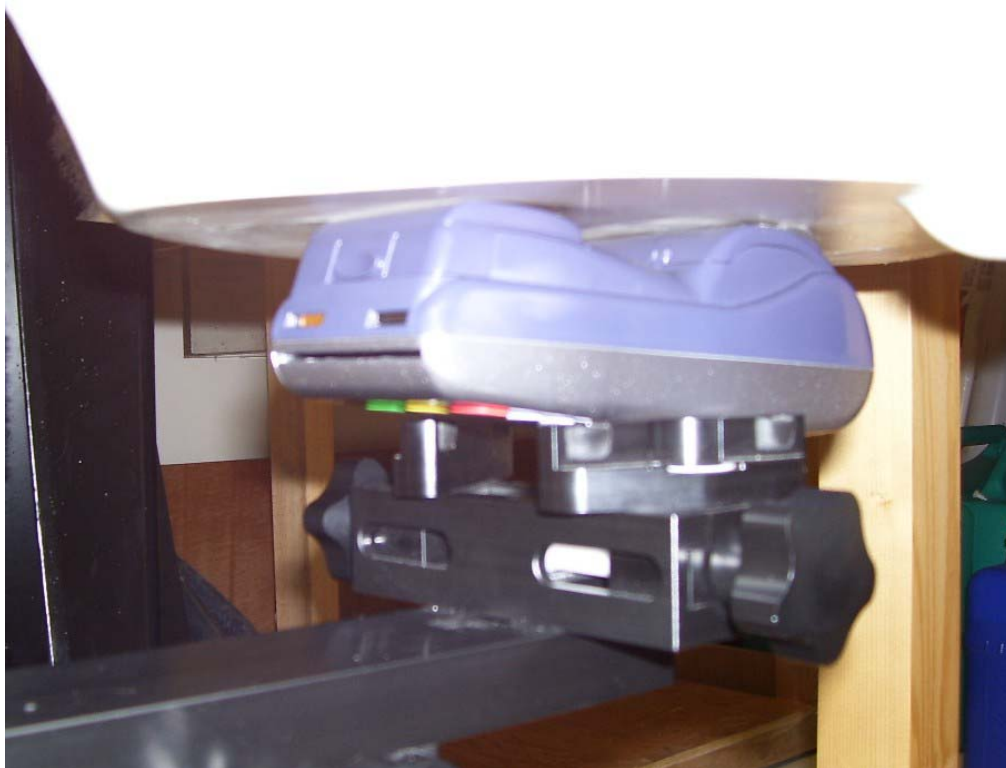
Back Side of EUT against Phantom with Battery Power
