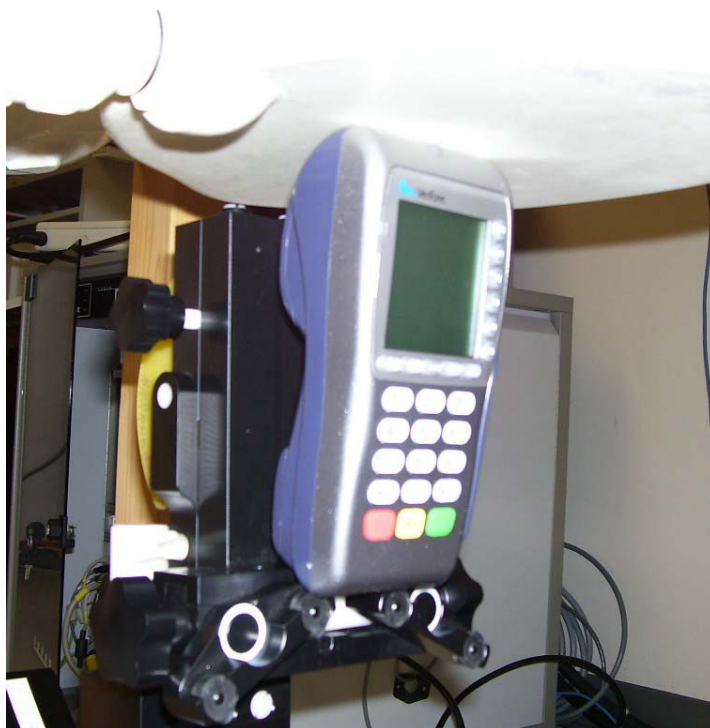
Antenna End of EUT against Phantom with Battery Power
