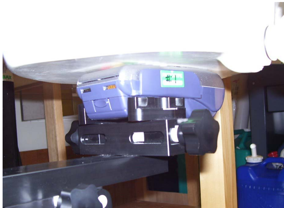
Front Side of EUT against Phantom with Battery Power
