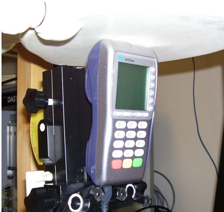
Antenna End of EUT against Phantom with External Power
