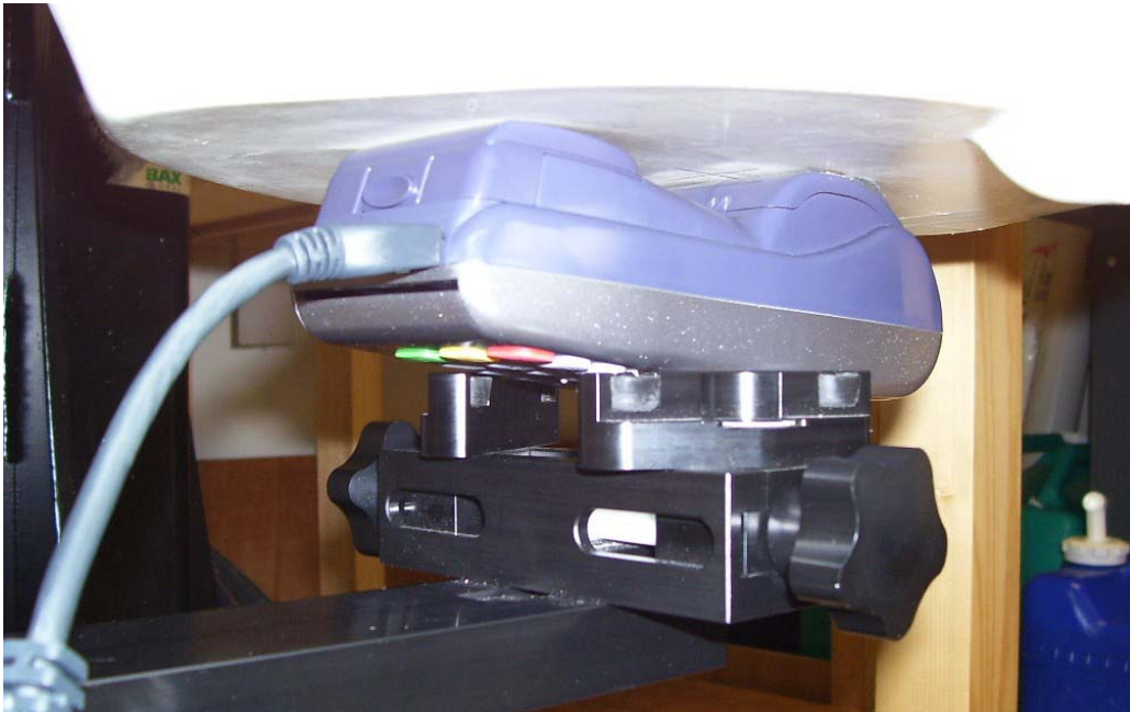
Back Side of EUT against Phantom with External Power
