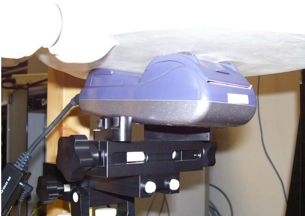
Back Side of EUT against Phantom with External Power
