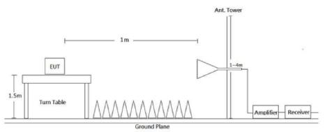
Radiated emission tests were performed in the 3 meters chamber test site, using the setup accordance with the ANSI C63.10-2013. The specification used was the FCC Part 15.209, FCC 15.247 Limits.
