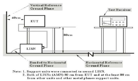
The setup of EUT is according with per ANSI C63.10-2013 measurement procedure. The specification used was with the FCC Part 15.207 limits.
