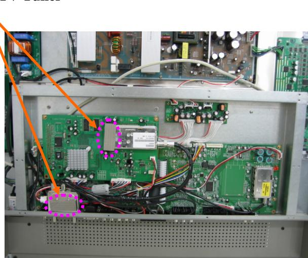
**3. Apply a ferrite Core to the Speaker cable and data cable**
