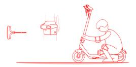
Please check whether the standpipe screw is loose first. If so, tighten the standpipe screw first, and then use a 6mm hex wrench to tighten the two screws of the folding mechanism. (If not, please contact your local dealer)
