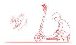
When replacing the griptape, please directly remove the surface sandpaper for replacement. Do not remove the PET board below the sandpaper.
