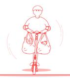
Do not hang heavy objects such as backpack on the handlebar as the stability of the vehicle can be affected.
