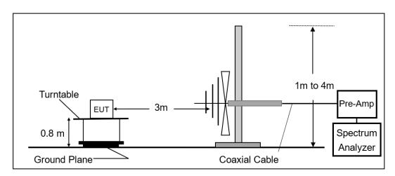
Radiated Emission Test Set-Up, Frequency Above 1GHz.
