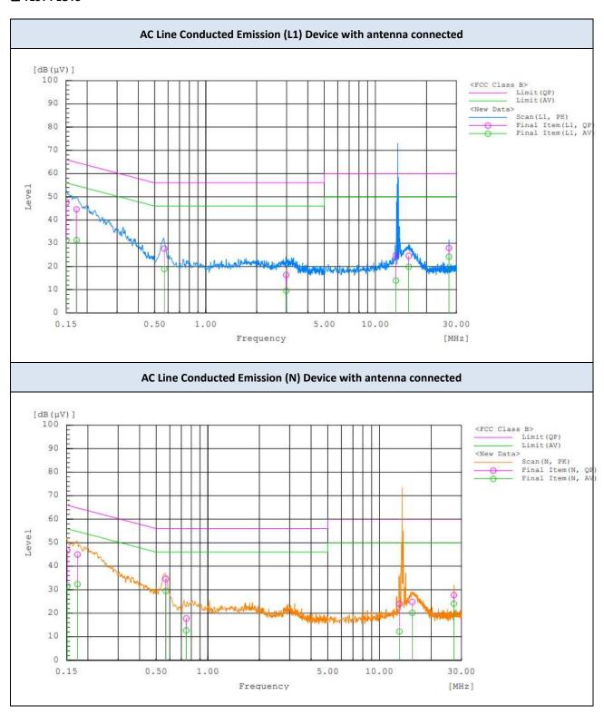
**Note**: Peak at 13.56 MHz is a fundamental frequency of HF.
