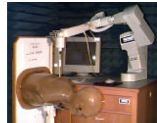
Fig. 1 SAR Test Setup
