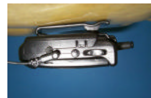
Figure 9. Body Holster Configuration
