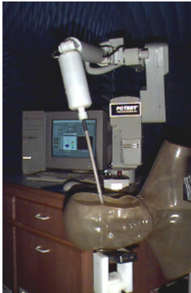
Figure 4. Photograph of the Probe and the Phantom
