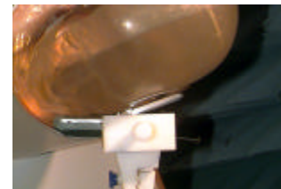
Fig. 11 Head SAR Test Setup
