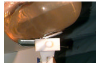
Fig. 10 Head SAR Test Setup
