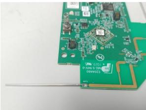
Photograph No.3 Wireless Transceiver Antenna assembly
