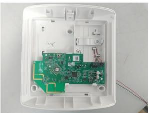
Photograph No.2 Wireless Transceiver Print side of the main PCB
