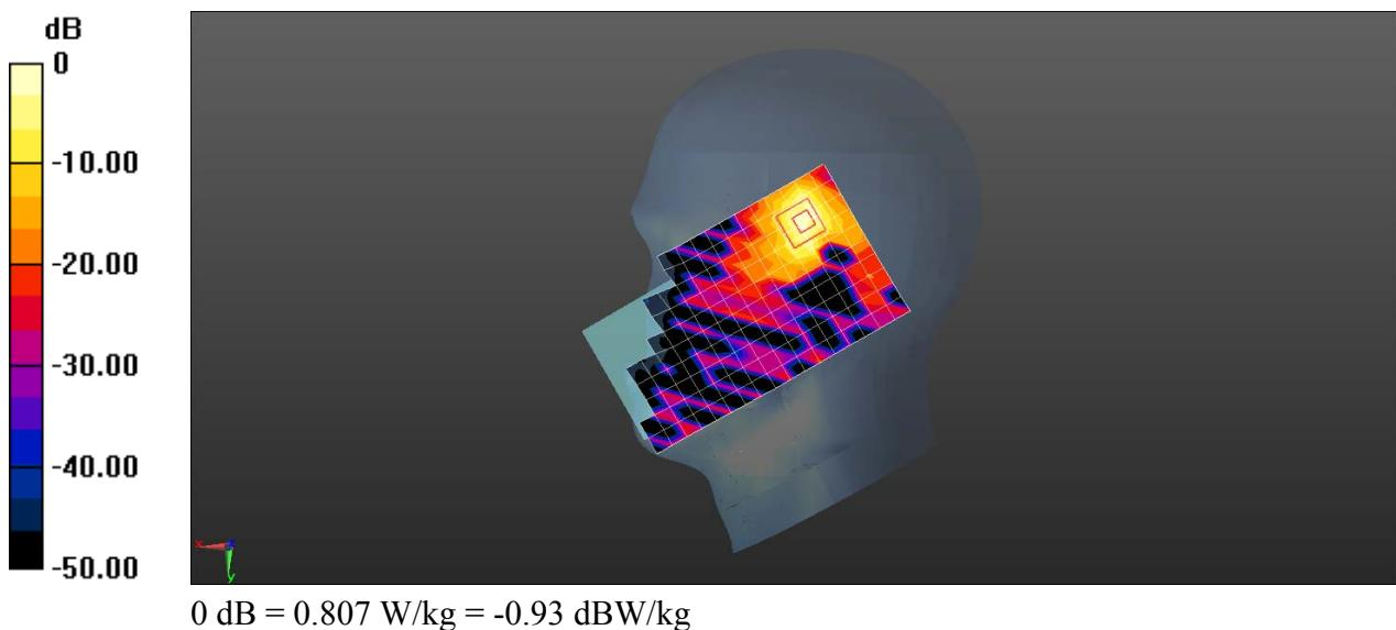
Test Laboratory: SGS-SAR Lab
