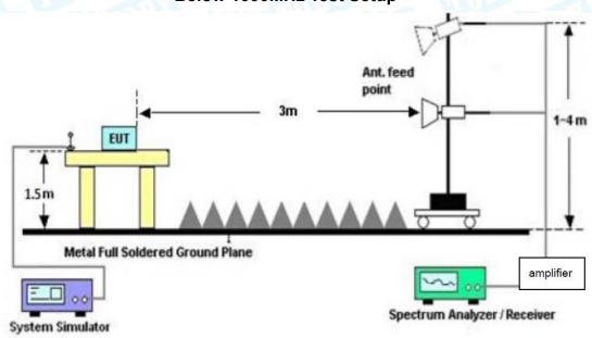
**Above 1GHz Test Setup**
