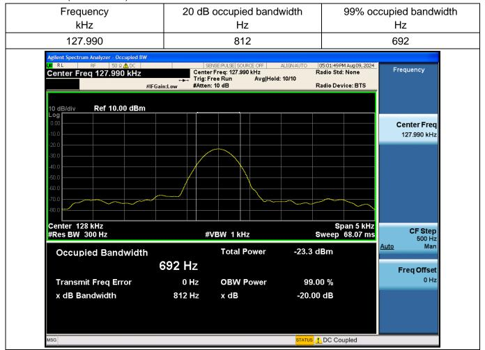
**Note:** Because the measured signal is CW-like, adjusting the RBW per C63.10 would not be practical since measurement bandwidth will always follow the RBW. The RBW is set to 300 Hz to perform the occupied bandwidth test.
