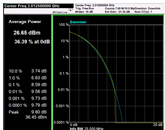
Channel: TOP, Modulation: 16QAM, BW=15MHz, CCDF
