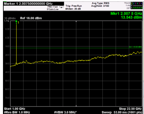
Channel: MIDDLE, Modulation: QPSK, BW=10MHz, Range: Upper
