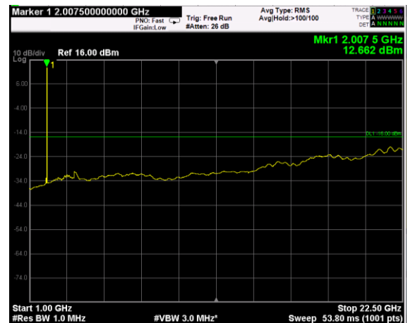
Channel: MIDDLE, Modulation: 64QAM, BW=5MHz, Range: Upper
