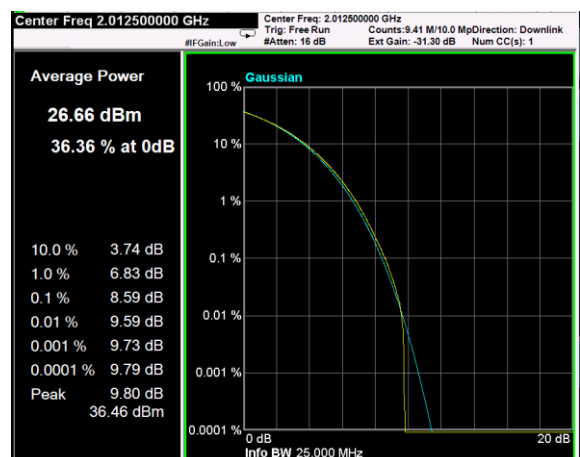
Channel: TOP, Modulation: 256QAM, BW=15MHz, CCDF
