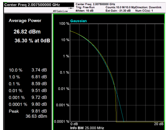
Channel: MIDDLE, Modulation: 64QAM, BW=15MHz, CCDF
