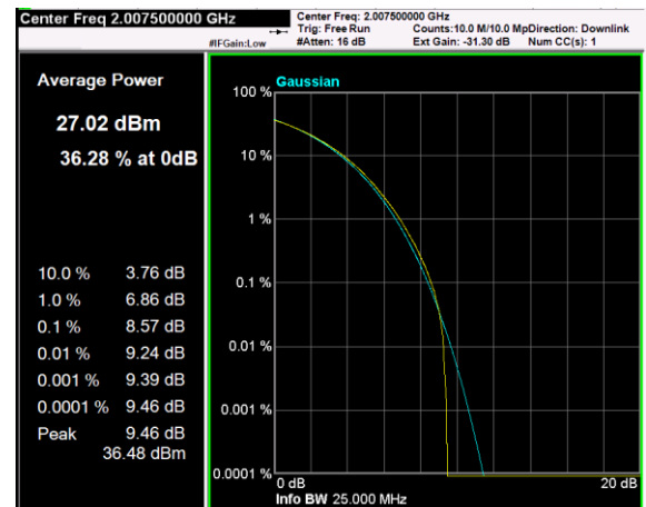
Channel: MIDDLE, Modulation: 256QAM, BW=20MHz, CCDF
