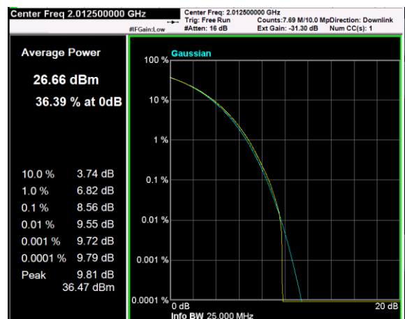
Channel: TOP, Modulation: QPSK, BW=15MHz, CCDF
