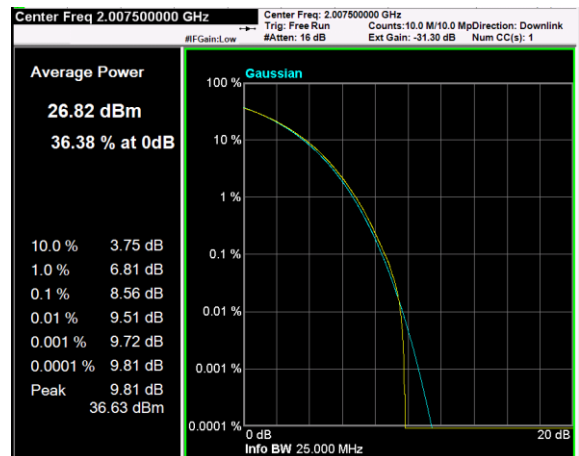
Channel: MIDDLE, Modulation: 16QAM, BW=15MHz, CCDF
