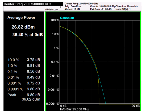
Channel: MIDDLE, Modulation: 256QAM, BW=15MHz, CCDF
