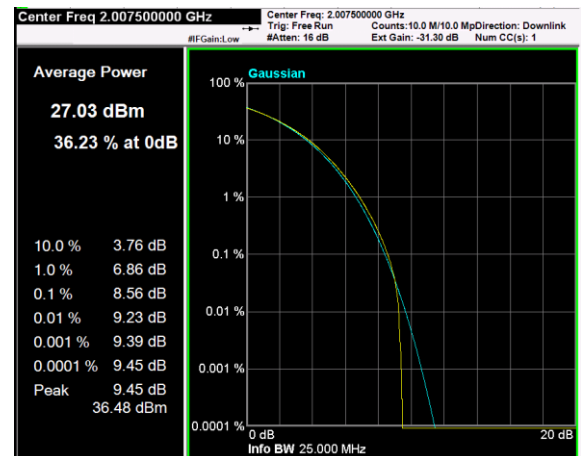
Channel: MIDDLE, Modulation: 16QAM, BW=20MHz, CCDF
