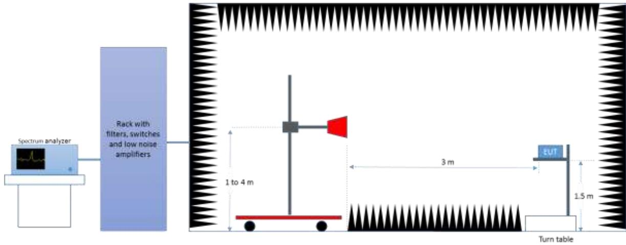
*Radiated Setup 6.4 GHz – 18 GHz*
