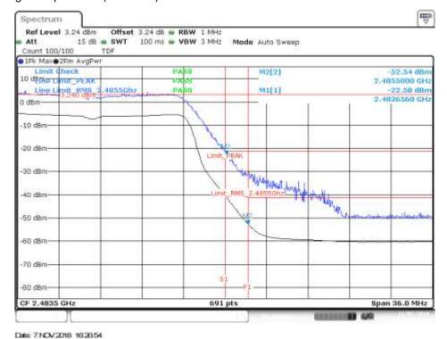
Channel 11 - BE High Freq Section RMS within 2MHz (restricted)
