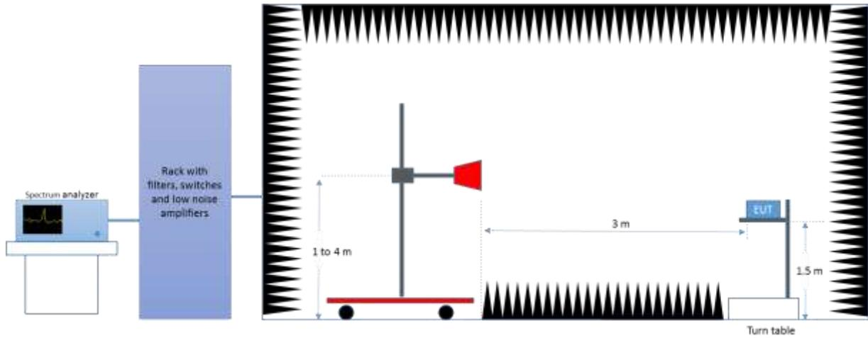
*Radiated Setup 1 GHz – 6.4 GHz (used for BLE tests)*
