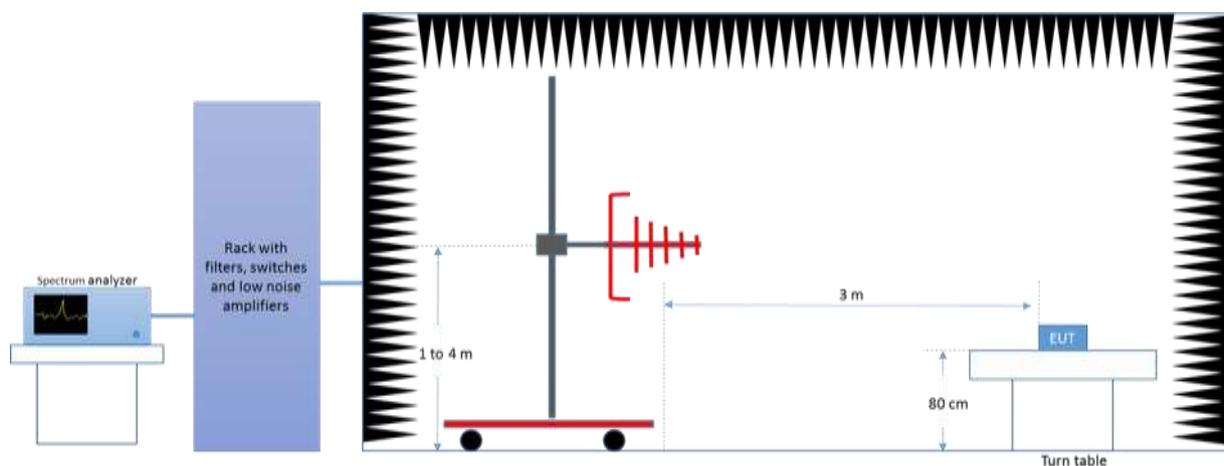
*Radiated Setup 1 GHz – 6.4 GHz ( used for DTS tests)*
