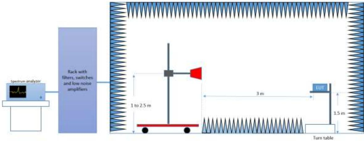
*Radiated Setup 6.4 GHz – 18 GHz*
