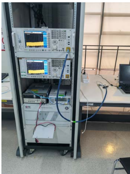
RF Conducted Test setup (BLE/WIFI)
