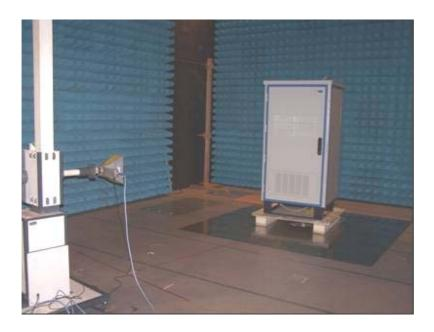
Radiated Emissions-Rear View (1) (above 1GHz)
