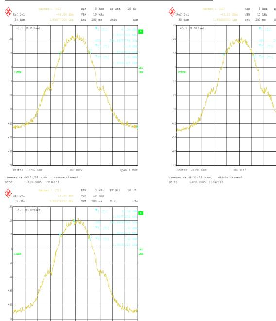
Note: The occupied bandwidth is measured using the internal OBW function of the measurement analyser. The analyser automatically configures the measurement bandwidths to make an accurate measurement. The results can be observed in the right hand corner of the graphs.
