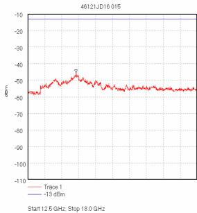
Start 12.5 GHz; Stop 18.0 GHz Ref-10 dBm; Ref Offset 28.0 dB; 10 dB/div RBW 1.0 MHz; VBW 1.0 MHz; Att 0 dB; Swp 40.0 mS Peak 14.071 GHz, -45.37 dBm Display Line: -13 dBm; 28/02/2005 21:24:11
