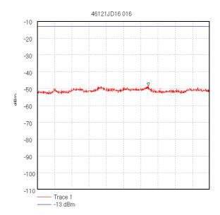
Start 18.0 GHz; Stop 20.0 GHz Ref -10 dBm; Ref Offset 31.2 dB; 10 dB/div RBW 1.0 MHz; VBW 1.0 MHz; Att 0 dB; Swp 20.0 mS Peak 19.289 GHz, -48.54 dBm Display Line: -13 dBm; 28/02/2005 21:28:17
