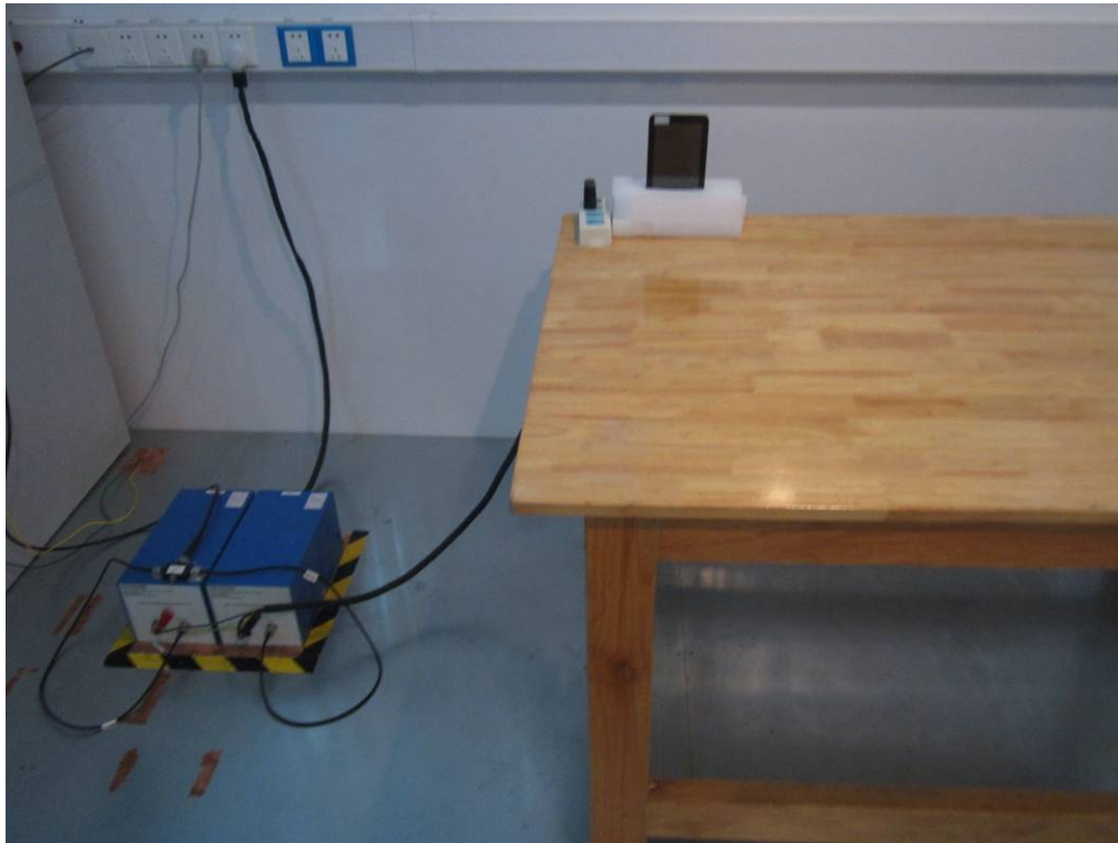
Conducted Emissions Test Setup Front View
