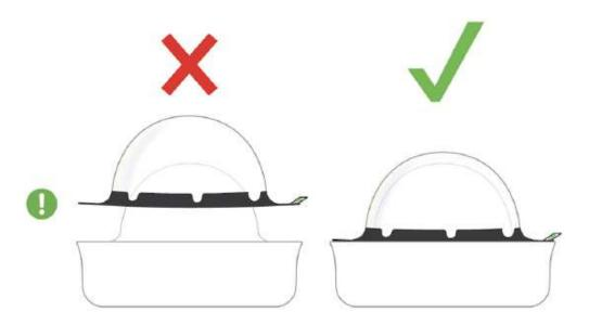
1. Carefully loosen all four Torx head security screws and remove the optical dome from the base. There is a tether cable attached to the optical dome and camera base to simplify installation. Remove the desiccant pack included in the camera during product shipment and replace with the provided spare desiccant pack. This is important to prevent moisture accumulating within the sealed optical dome.
