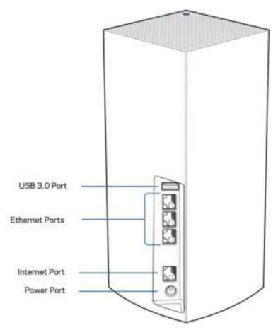
USB 3.0 port— Connect and share USB drives on your network. For local file sharing only (no FTP, media server or virtualUSB support). Also, not intended for sharing peripherals such as printers, scanners or cameras.
