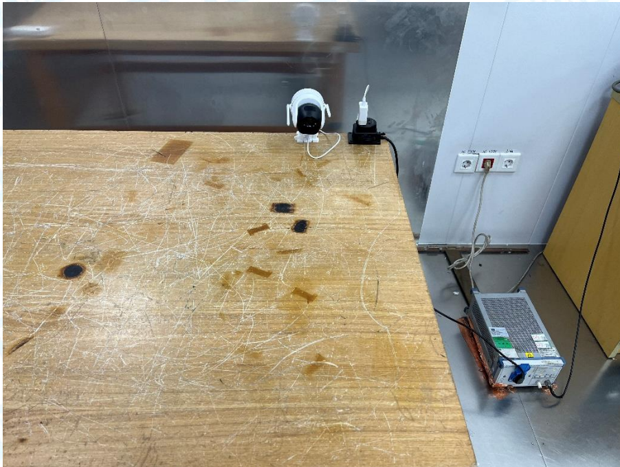
Photo of Setup for Radiated Emission (30MHz~1GHz)
