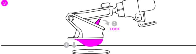
Remove the plastic cover from the suction cup and firmly press onto the dashboard pad. Push the lever down to engage suction.
