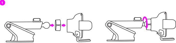
Connect the mount cradle to the ball joint. Tighten the cradle knob.
