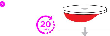
Choose a flat mounting location on your dashboard and wipe the surface clean. Peel off the film on the dashboard pad and evenly press onto the desired location. Wait 20 minutes.
