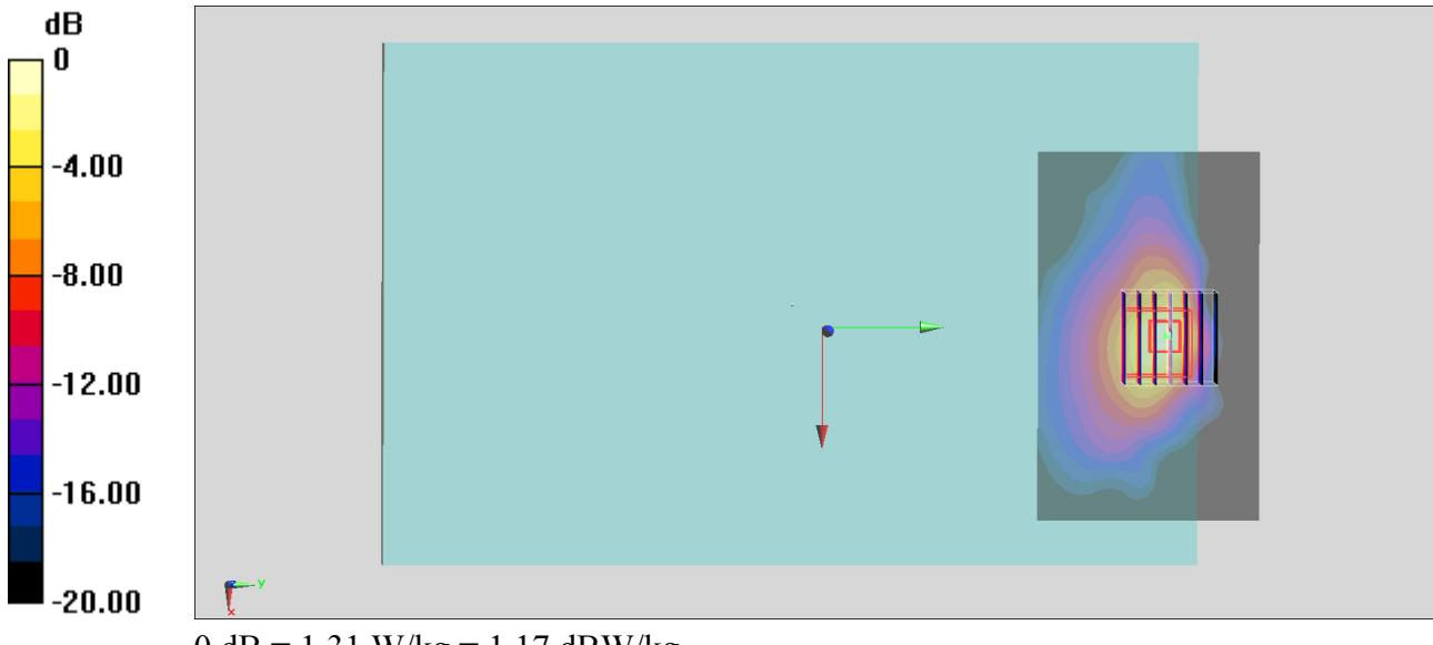
**#02\_WLAN5GHz\_802.11ac-VHT80 MCS0\_Bottom Face\_0mm\_Ch58;Ant 1**
