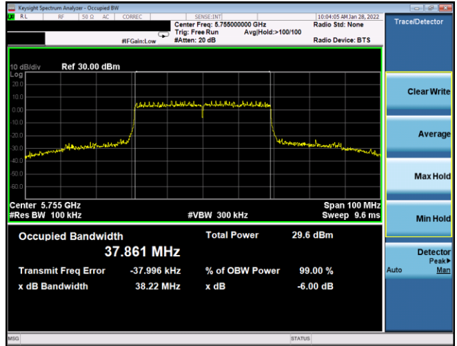
Plot 7-136. 6dB BW & 99% OBW Antenna WF7a (40MHz BW 802.11ax (SU) – Ch. 151, MCS3)
