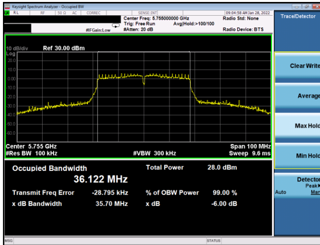
Plot 7-111. 6dB BW & 99% OBW Antenna WF8 (40MHz BW 802.11n – Ch. 151, MCS0)
