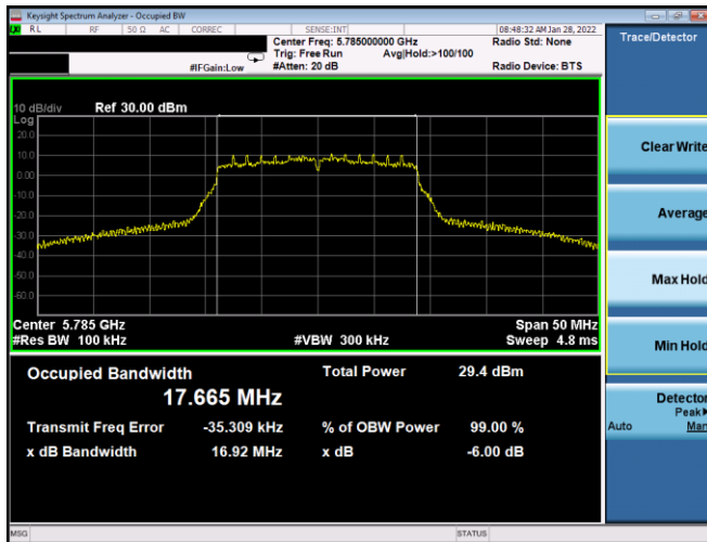
Plot 7-109. 6dB BW & 99% OBW Antenna WF8 (20MHz BW 802.11n – Ch. 157, MCS0)
