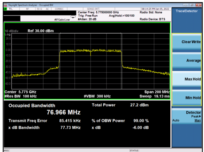
Plot 7-126. 6dB BW & 99% OBW Antenna WF8 (80MHz BW 802.11ax(SU) – Ch. 155, MCS5)
