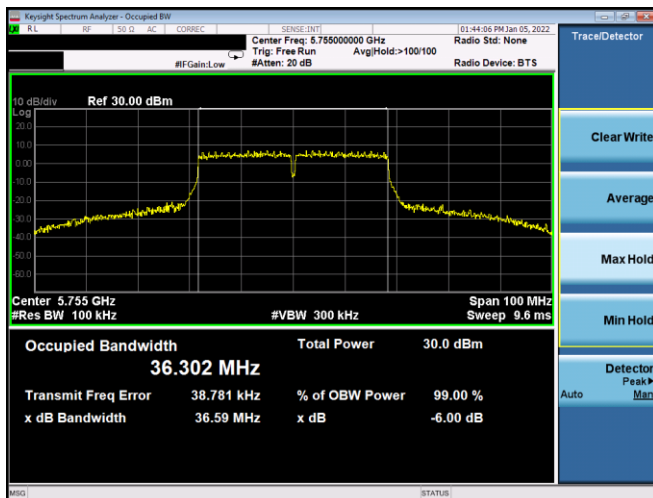
Plot 7-123. 6dB BW & 99% OBW Antenna WF8 (40MHz BW 802.11n – Ch. 151, MCS5)
