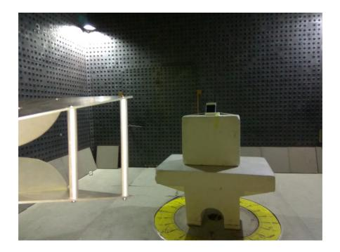
Photograph No.4 Setup for spurious emission at receiver port
