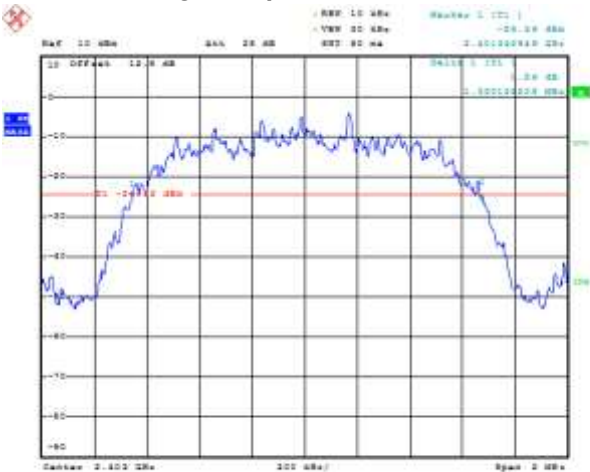
Figure 5-4: 20 dB Bandwidth Single freq. CH 0 Static PBRS, 2-DH5
