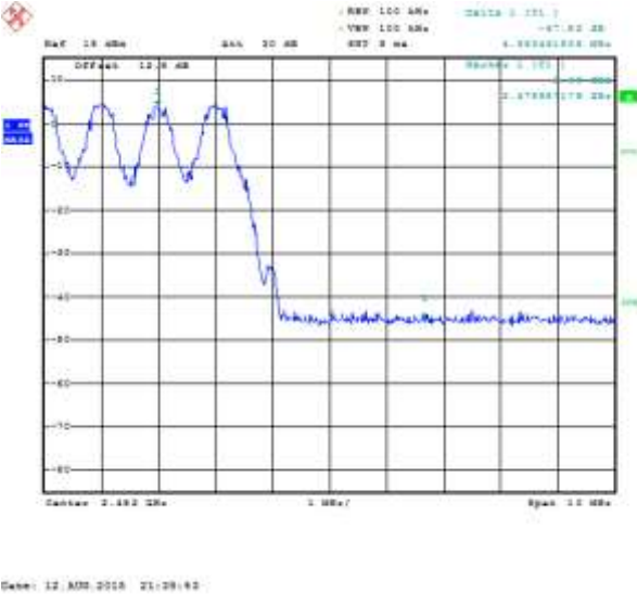
Figure 5-29: Band Edge Compliance Freq. Hopping, Static PBRS, DH5
