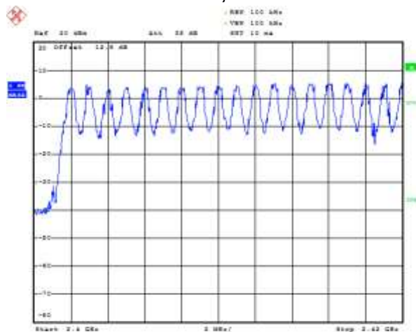
Figure 5-13: Number of Hopping Frequencies Static PBRS, DH5
