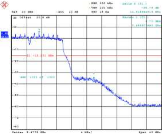
Figure 6-24: Band Edge Compliance Primary, 802.11n, Channel 11, MCS 0
