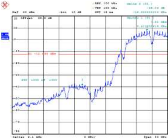
Figure 6-19: Band Edge Compliance Primary, 802.11b, Channel 1, 1 Mbps
