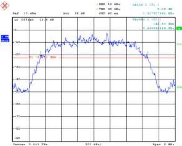
Figure 5-5: 20 dB Bandwidth Single freq. CH 39 Static PBRS, 2-DH5
