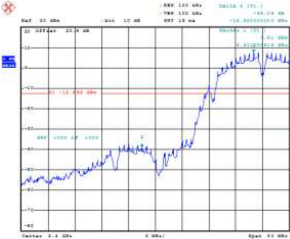
Figure 6-19: Band Edge Compliance Secondary, 802.11b, Channel 1, 1 Mbps
