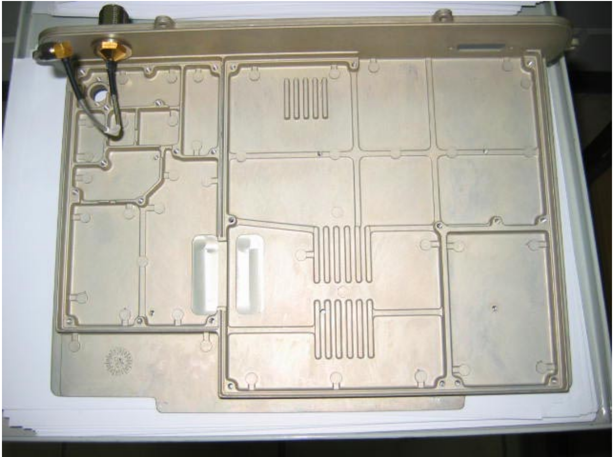
Photograph No.16 SPR 700MHz internal view
