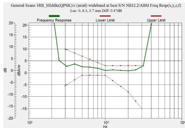
Figure C.14 Frequency Response of LTE B41 Power Class 2
