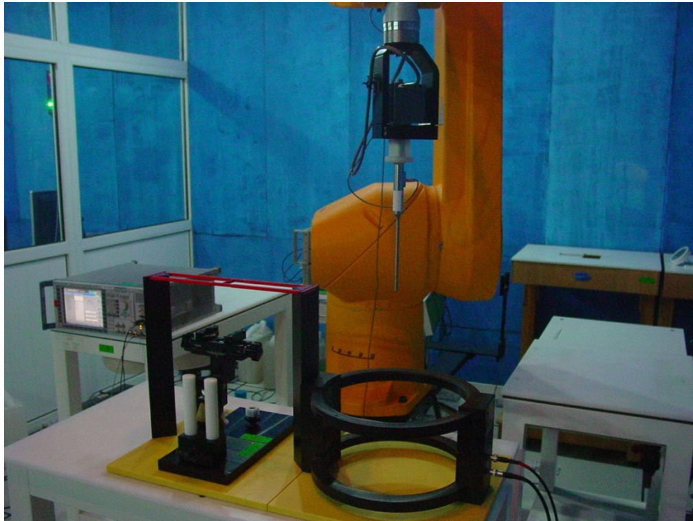
Picture A1: HAC T-Coil System Layout
