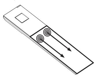
3. Lift the battery cover off the handset.
