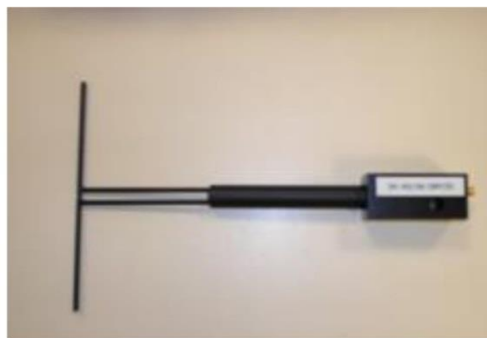
Figure 1 – Satimo COMOSAR Validation Dipole
