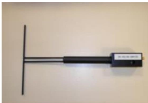
Figure 1 – Satimo COMOSAR Validation Dipole
