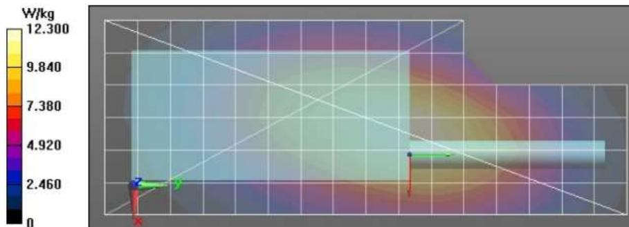
Shortened scan reflects highest SAR producing configuration and is compared to the full scan.
