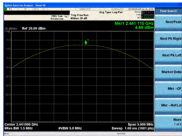
Peak output Power plot on channel 39 (2Mbps)
