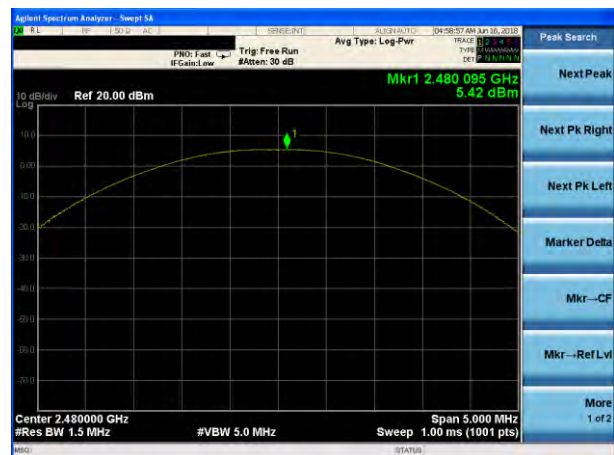
Peak output Power plot on channel 78 (2Mbps)
