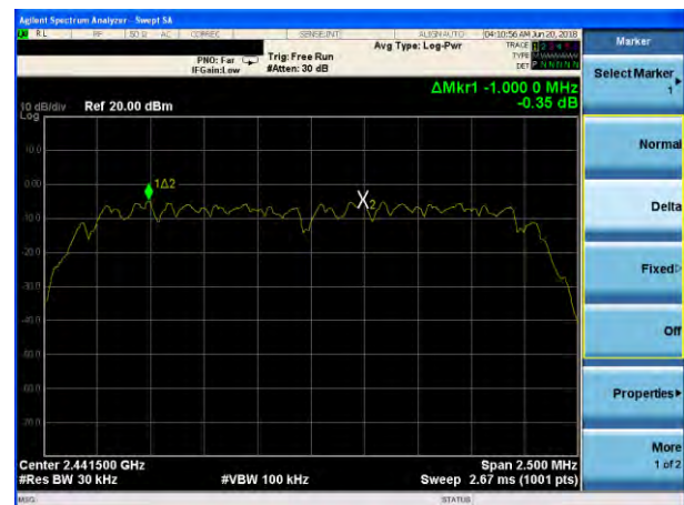
(2Mbps) Channel Separation plot on channel 39-40
