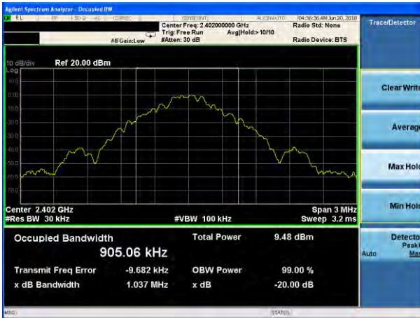
20dB Bandwidth plot on channel 39 (1Mbps)
