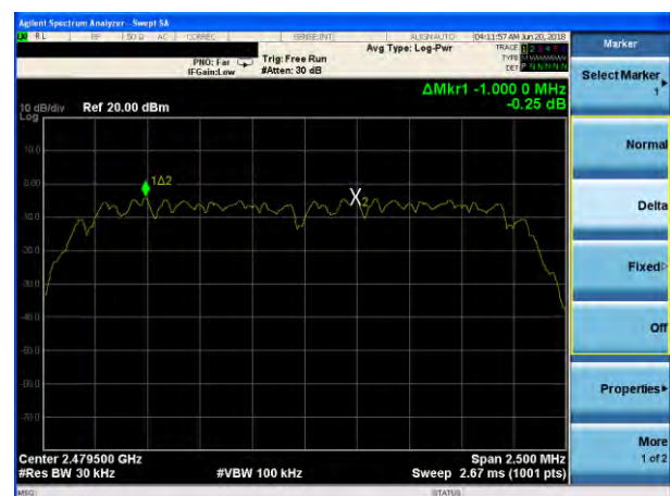
(2Mbps) Channel Separation plot on channel 77-78
