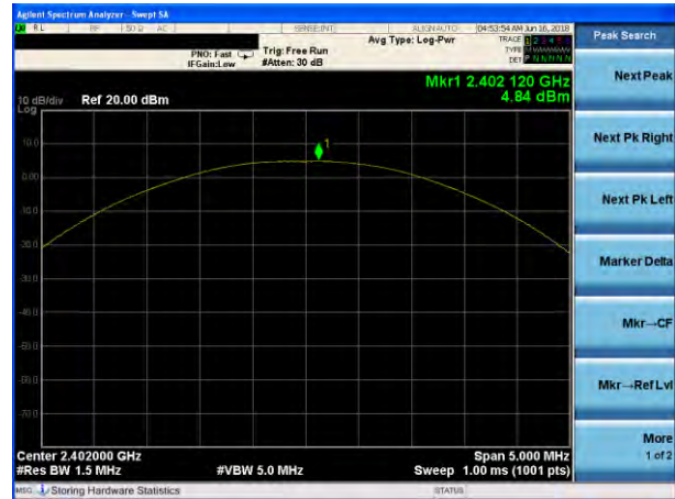
Peak output Power plot on channel 39 (2Mbps)
