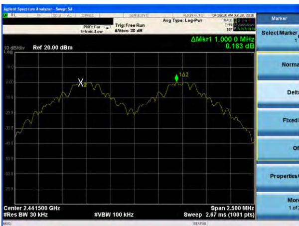
(1Mbps) Channel Separation plot on channel 39-40
