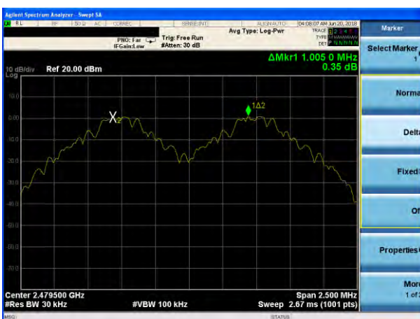
(1Mbps) Channel Separation plot on channel 77-78
