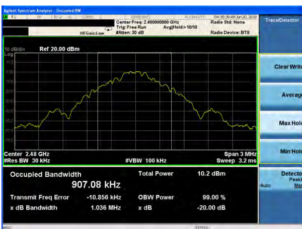
20dB Bandwidth plot on channel 78 (1Mbps)
