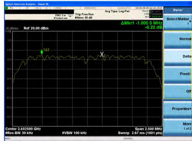
(2Mbps) Channel Separation plot on channel 39-40
