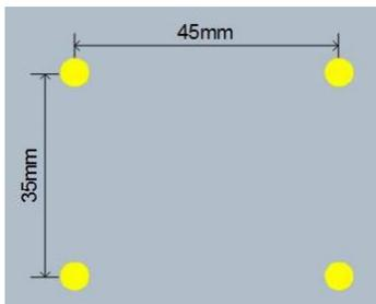
3. Drill four 10mm diameter and 70mm depth holes in the wall by following the marked locations.
