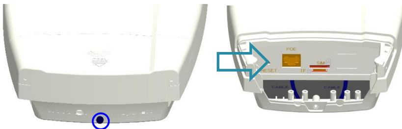
2. Insert the USIM card to the USIM slot. Note following the directions.
