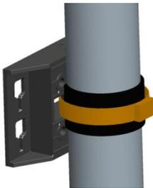
3. Install the CPE to the bracket and fasten the screw.
