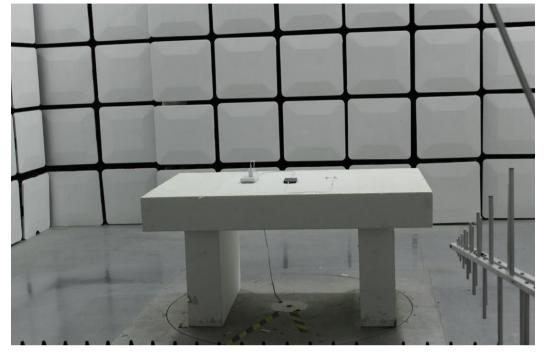
**1.3** Setup for Unwanted Emissions that fall Outside of the Restricted Bands(Radiated) and Unwanted Emissions in the Restricted Bands (Radiated) above 1GHz
