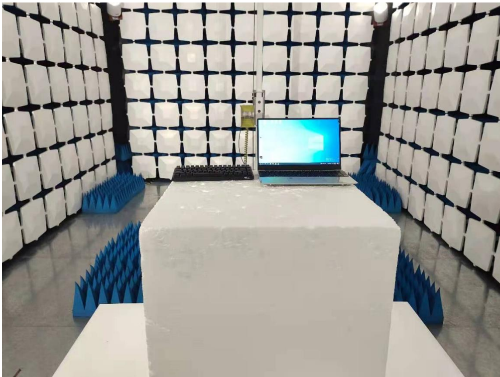
Above 1GHz for radiated emission test setup
