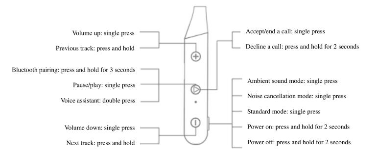
Mode switch: Press the power button to switch amongst the Ambient sound mode/Noise cancellation mode/Standard mode;
