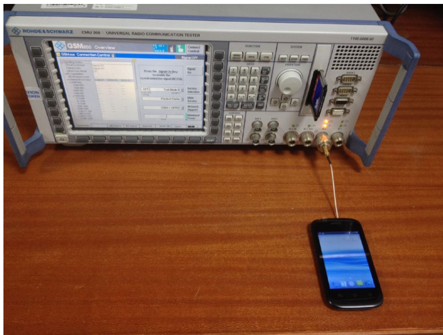
Photograph –2G&3G Conducted Test Setup
