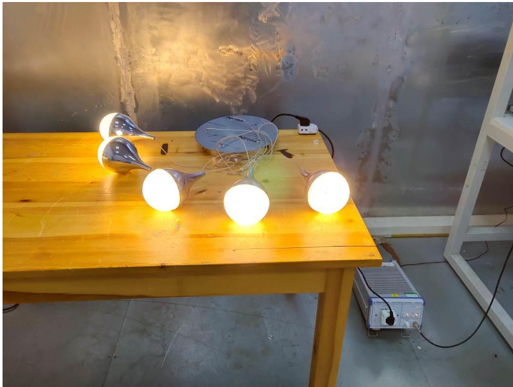
Photo of Power Line Conducted Measurement
