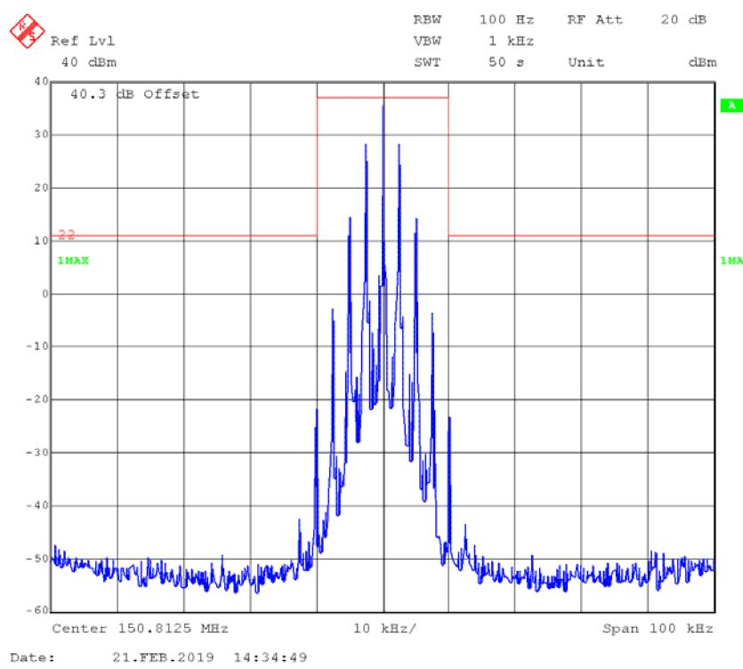
**FM,12.5kHz,Low Power - Frequency 150.8125 MHz: 99% Occupied & 26 dB Bandwidth**
