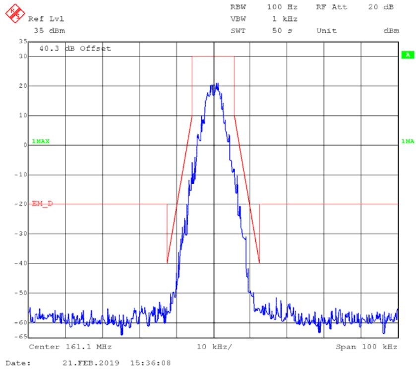
**Part 22****FM,12.5kHz,High Power - Frequency 150.8125 MHz: 99% Occupied & 26 dB Bandwidth**
