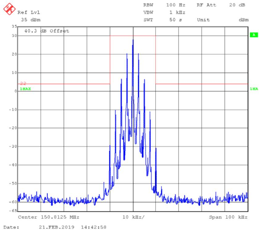
**FM,25kHz,High Power - Frequency 150.8125 MHz: 99% Occupied & 26 dB Bandwidth**
