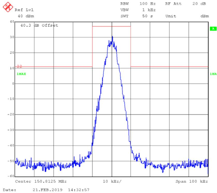
**4FSK,12.5kHz,Low Power - Frequency 150.8125 MHz: 99% Occupied & 26 dB Bandwidth**
