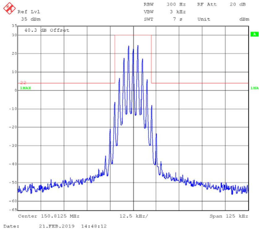
**4FSK,12.5kHz,High Power - Frequency 150.8125 MHz: 99% Occupied & 26 dB Bandwidth**
