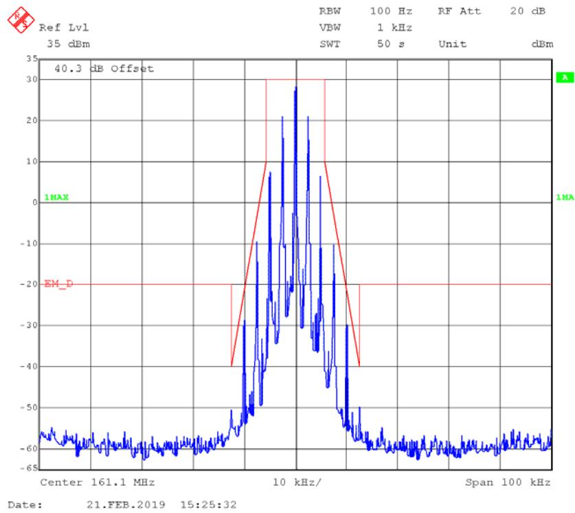
**FM,25kHz,High Power - Frequency 161.1 MHz: 99% Occupied & 26 dB Bandwidth**
