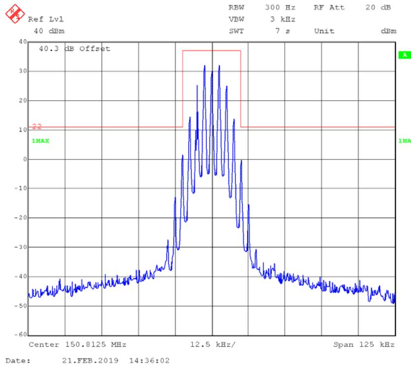
**FM,25kHz,Low Power - Frequency 150.8125 MHz: 99% Occupied & 26 dB Bandwidth**
