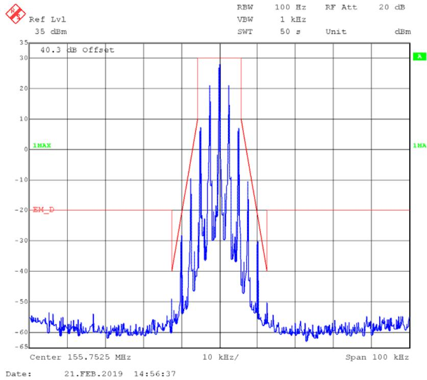
**4FSK,12.5kHz,High Power - Frequency 155.7525 MHz: 99% Occupied & 26 dB Bandwidth**
