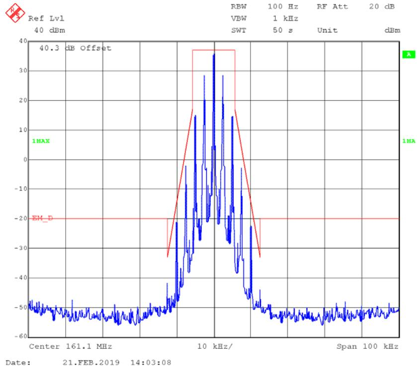
**FM,12.5kHz,Low Power - Frequency 161.1 MHz: 99% Occupied & 26 dB Bandwidth**
