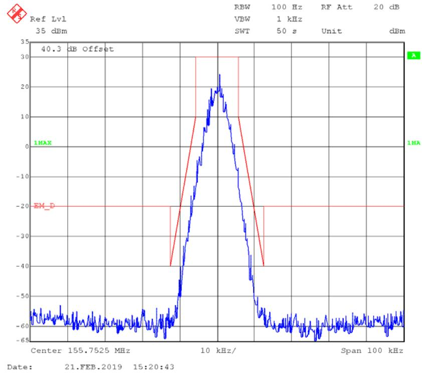
**Part 74****FM,12.5kHz,High Power - Frequency 161.1 MHz: 99% Occupied & 26 dB Bandwidth**
