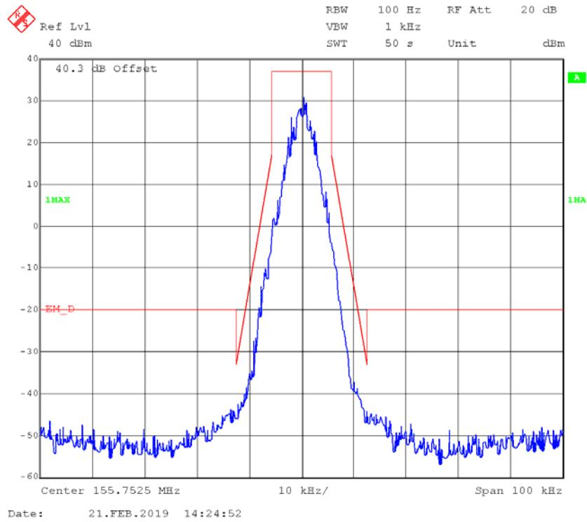
**4FSK,12.5kHz,Low Power - Frequency 155.7525 MHz: 99% Occupied & 26 dB Bandwidth**
