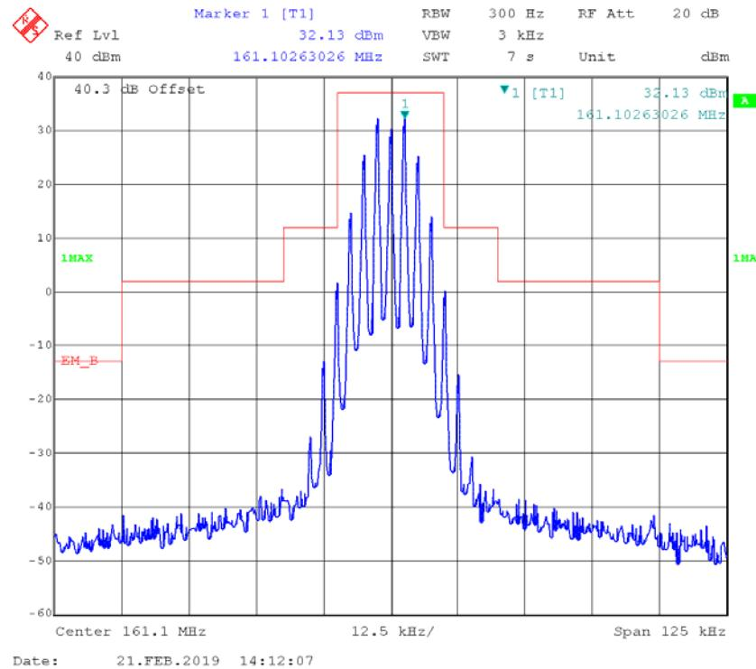
**FM,25kHz,Low Power - Frequency 161.1 MHz: 99% Occupied & 26 dB Bandwidth**
