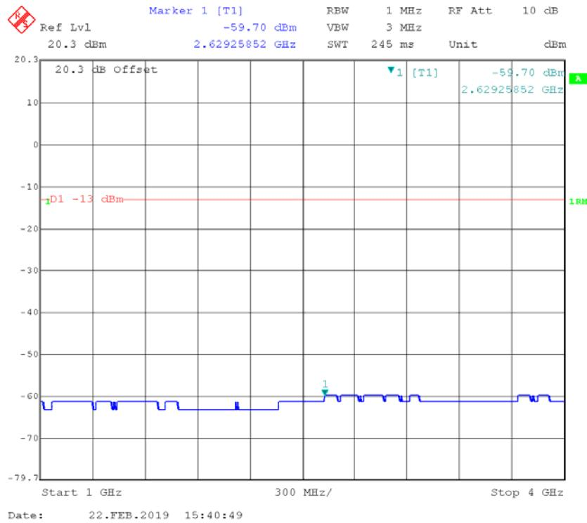
**12.5kHz, 4FSK, High power:****30MHz – 1 GHz, Channel Spacing 12.5 kHz, 161.1 MHz**
