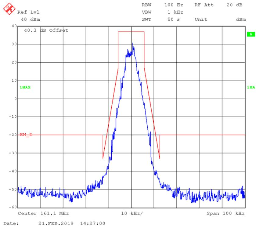
**4FSK,12.5kHz,Low Power - Frequency 161.1 MHz: 99% Occupied & 26 dB Bandwidth**
