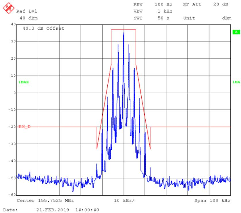
**FM,12.5kHz,Low Power - Frequency 155.7525 MHz: 99% Occupied & 26 dB Bandwidth**
