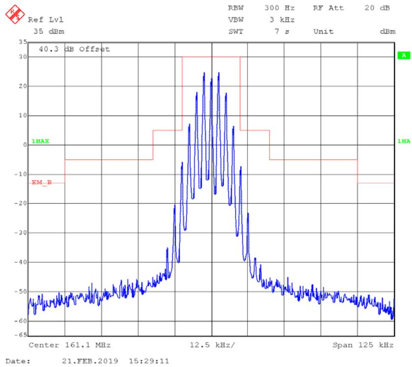
**4FSK,12.5kHz,High Power - Frequency 161.1 MHz: 99% Occupied & 26 dB Bandwidth**
