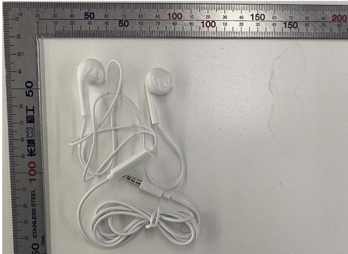
Headset (DEM-8A made by Shenzhen FDC Electronics Co.,Ltd)
