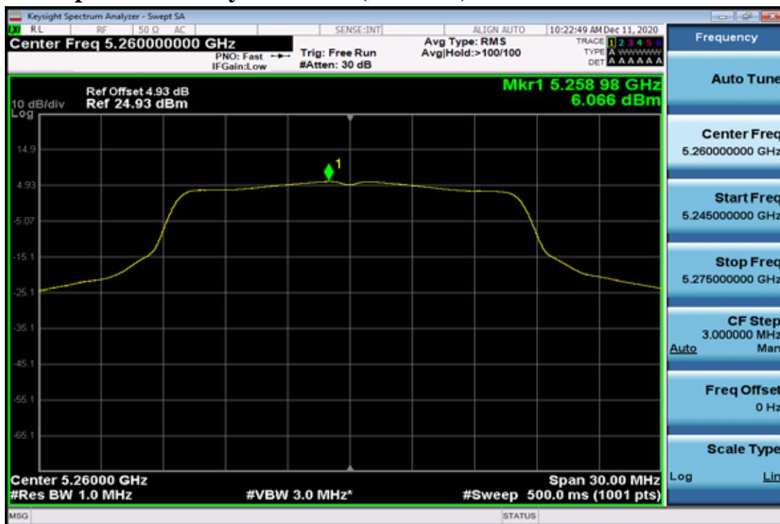
**Power Spectral Density Data Plot (CH Mid)**
