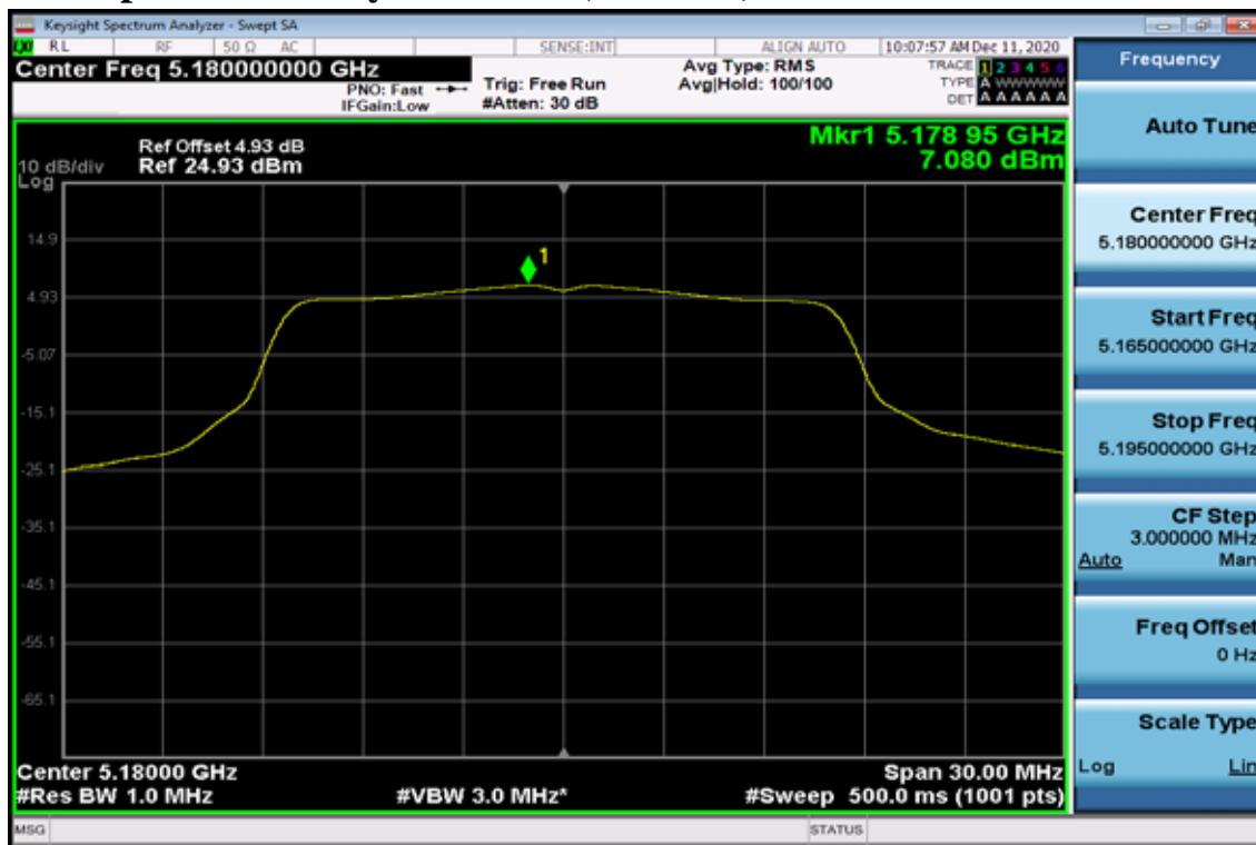
**Power Spectral Density Data Plot (CH Mid)**
