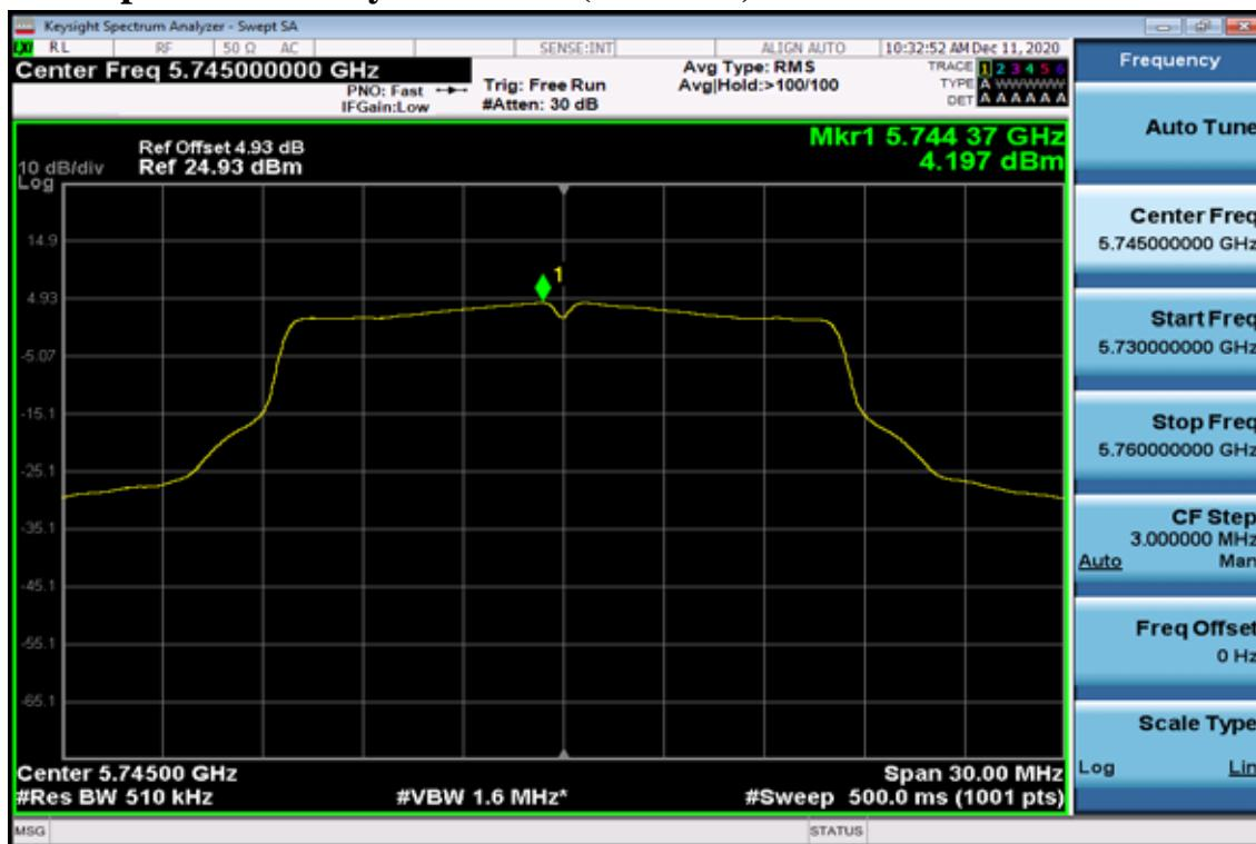
**Power Spectral Density Data Plot (CH Mid)**
