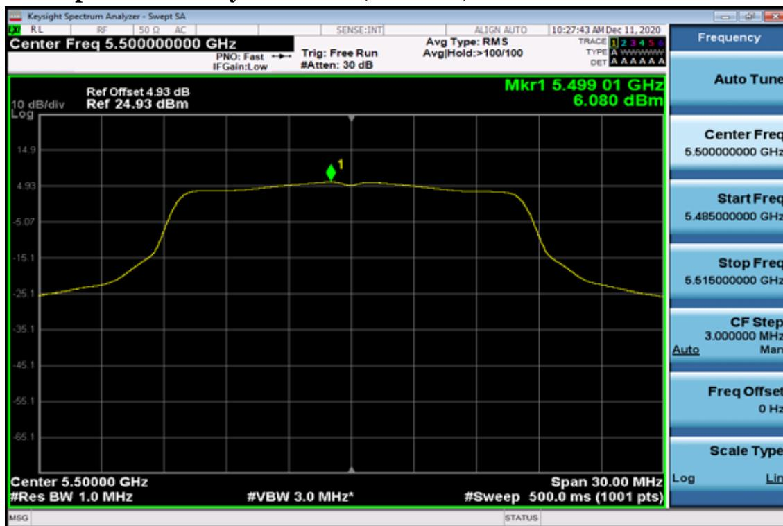
**Power Spectral Density Data Plot (CH Mid)**
