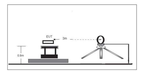
(B) Radiated Emission Test Set-Up Frequency Below 1 GHz
