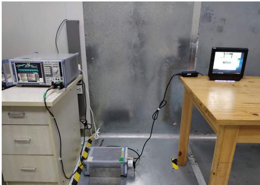
Radiated Spurious Emissions From 30MHz-1000MHz
