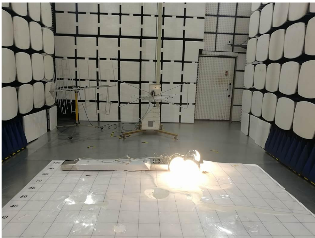
Photo of Radiated Measurement
