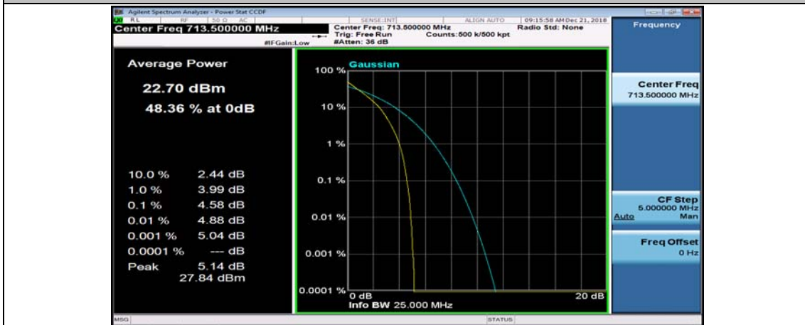
(Channel Bandwidth: 5 MHz)_HCH_QPSK_12RB#6
