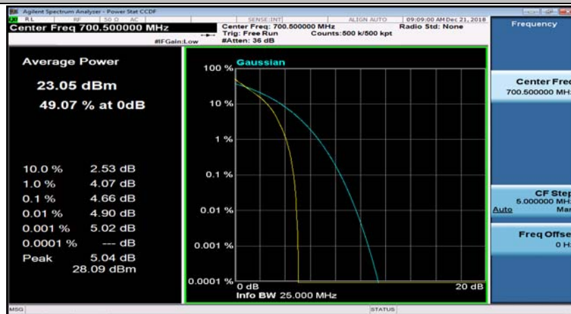
(Channel Bandwidth: 3 MHz)_LCH_QPSK_8RB#7
