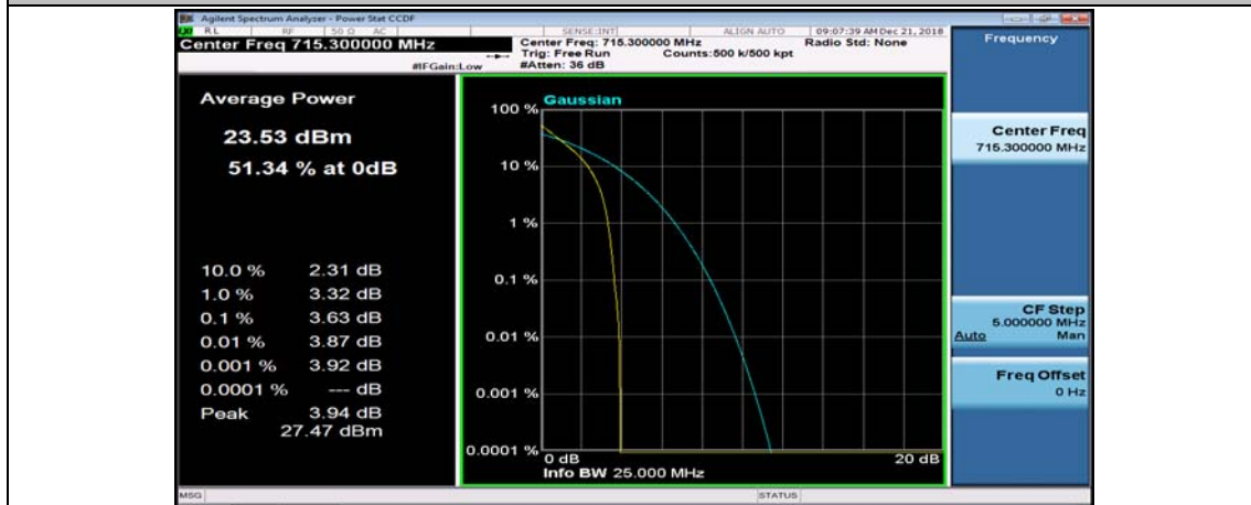
(Channel Bandwidth: 1.4 MHz)_HCH_QPSK_6RB#0
