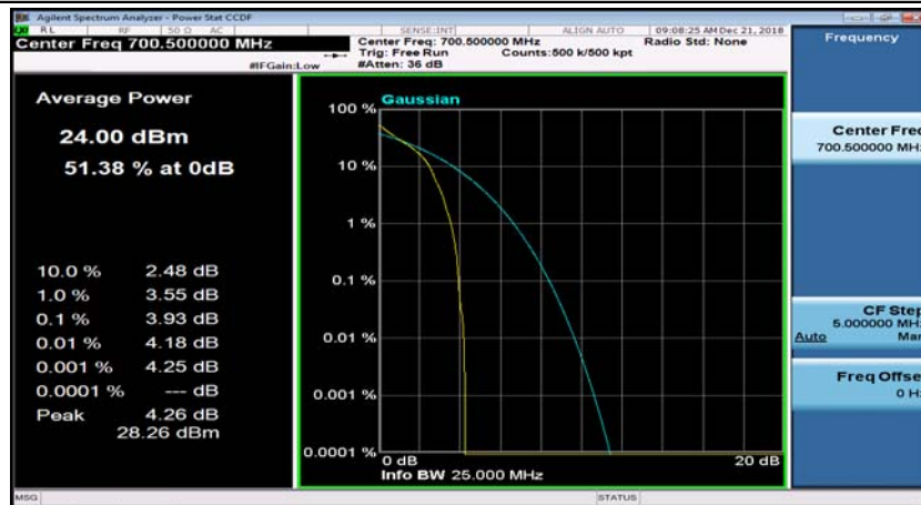
(Channel Bandwidth: 3 MHz)_LCH_QPSK_1RB#14
