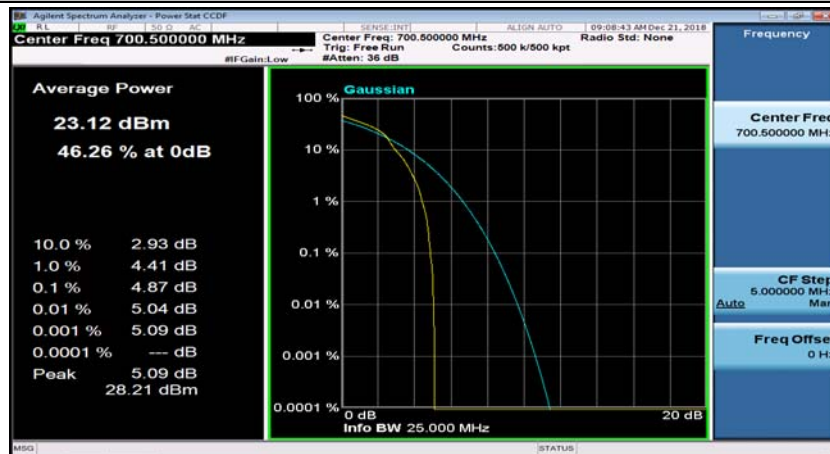
(Channel Bandwidth: 3 MHz)_LCH_16QAM_1RB#14
