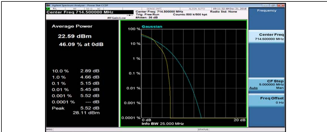
(Channel Bandwidth: 3 MHz)_HCH_16QAM_1RB#14
