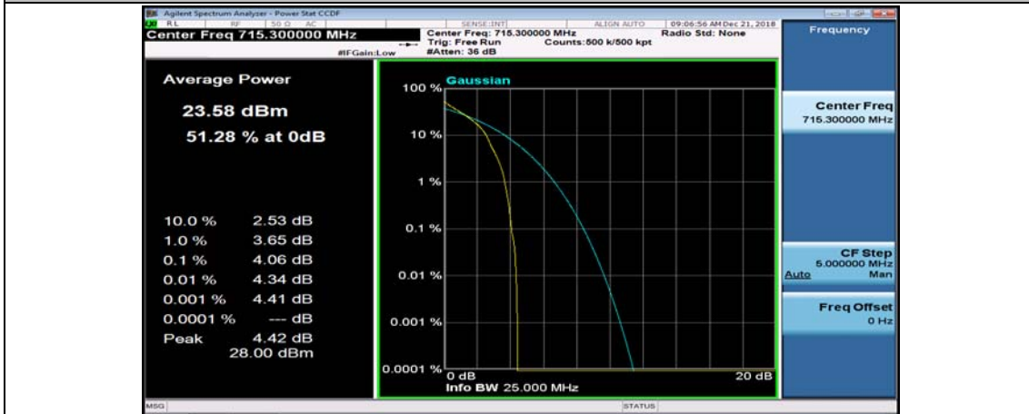
(Channel Bandwidth: 1.4 MHz)_HCH_QPSK_1RB#3
