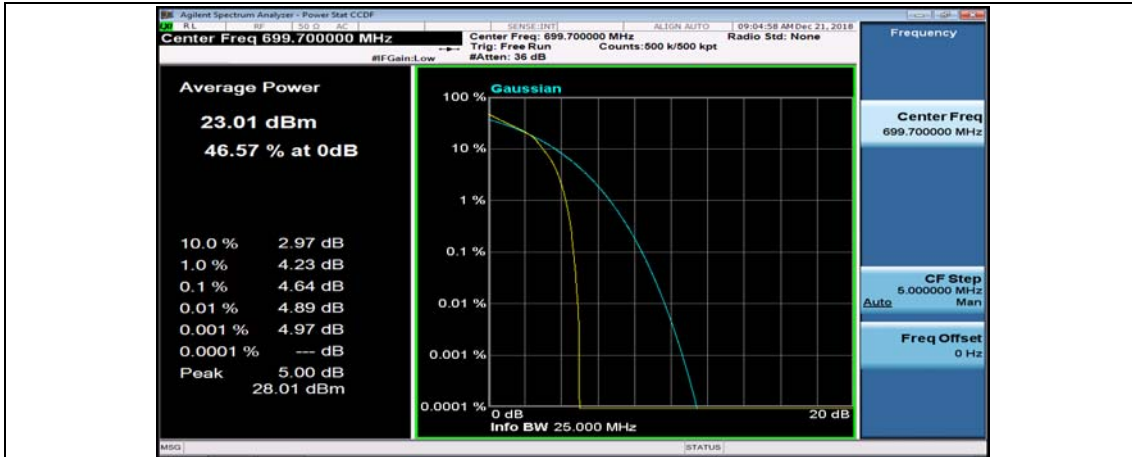
(Channel Bandwidth: 1.4 MHz)_LCH_16QAM_3RB#2
