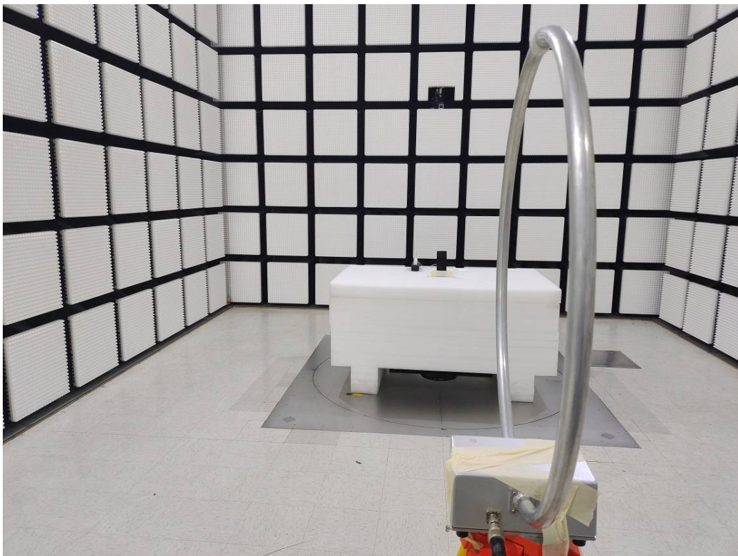
Radiated Emission Below 30MHz View Perpendicular
