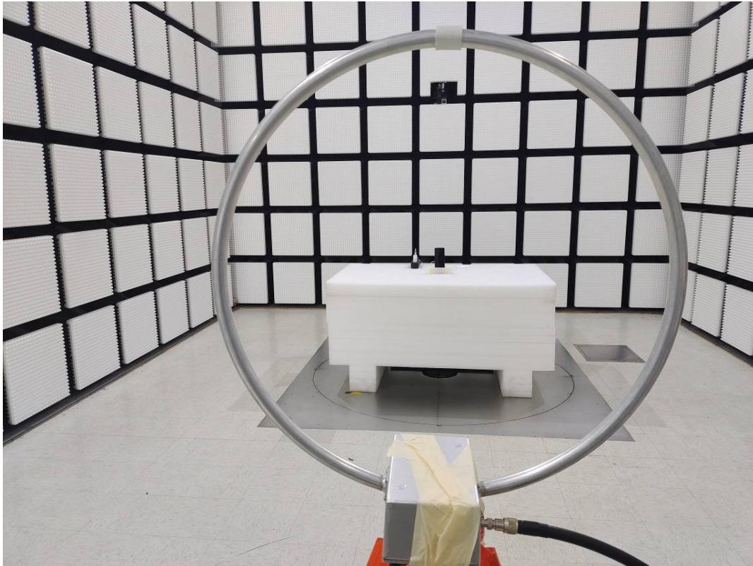
Radiated Emission Below 30MHz View Perpendicular
