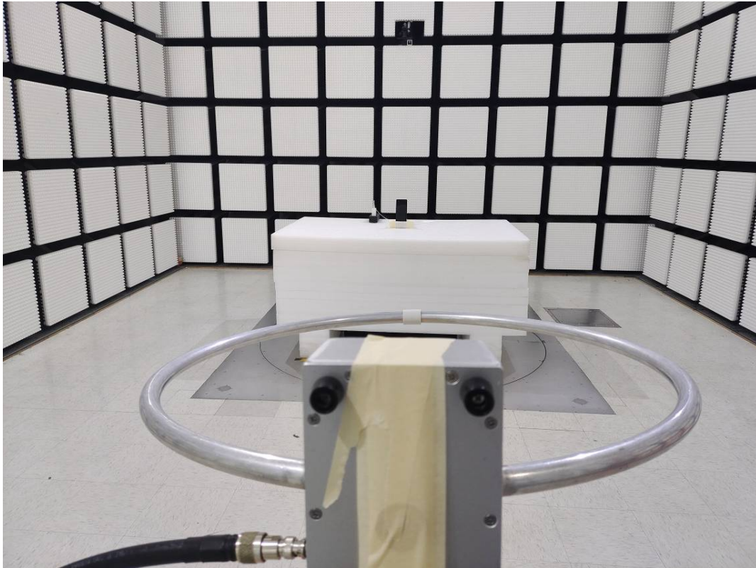
Radiated Emission Below 1GHz View
