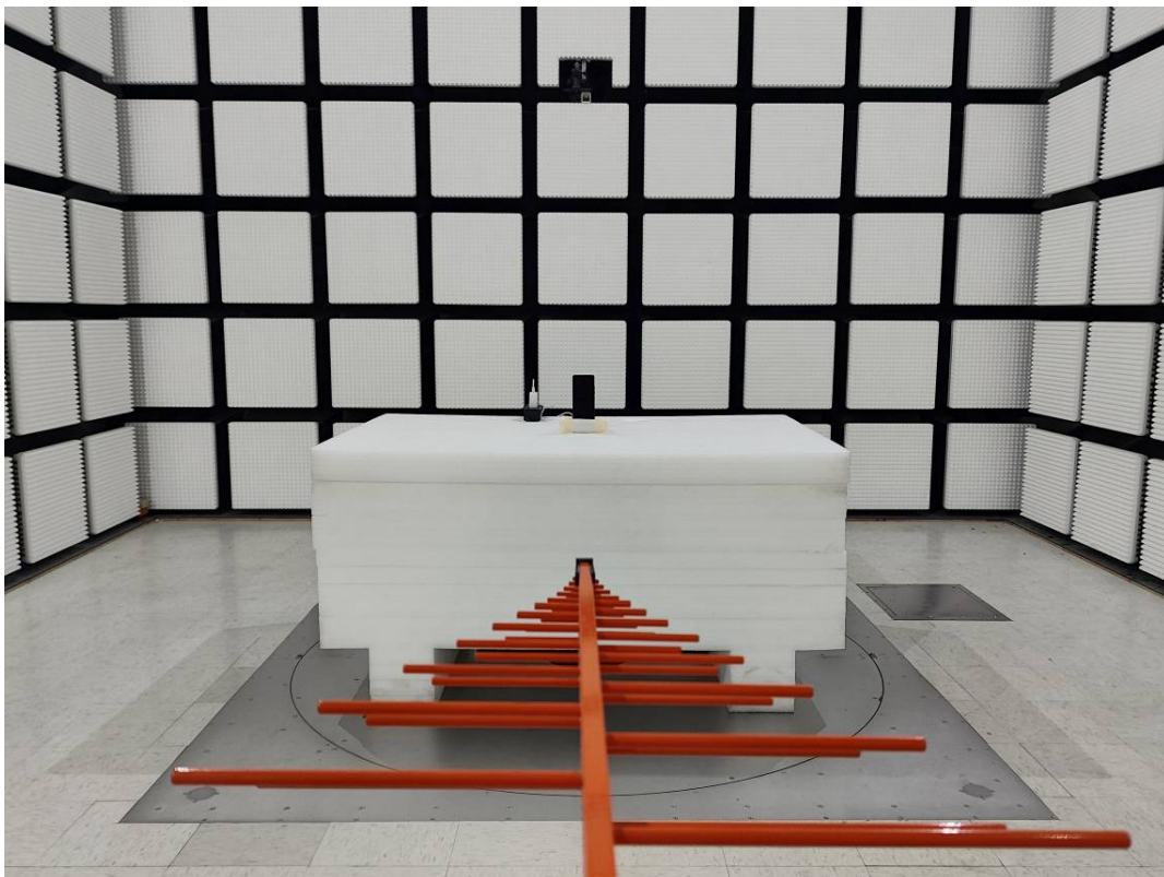
Radiated Emission Below 1GHz View
