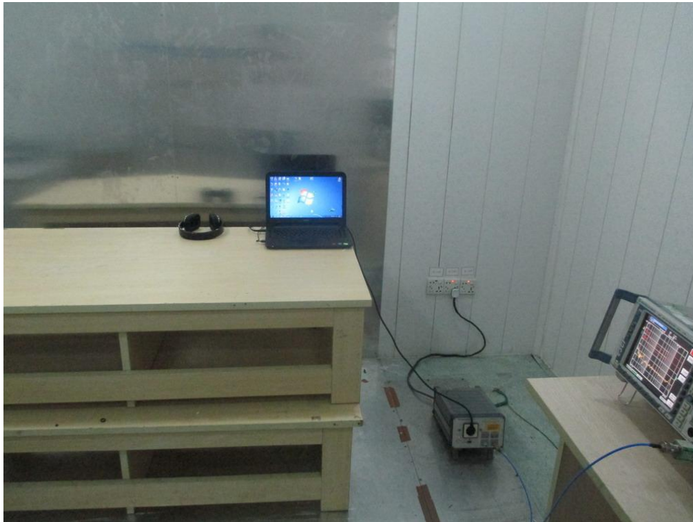
FCC RADIATED EMISSION TEST SETUP
