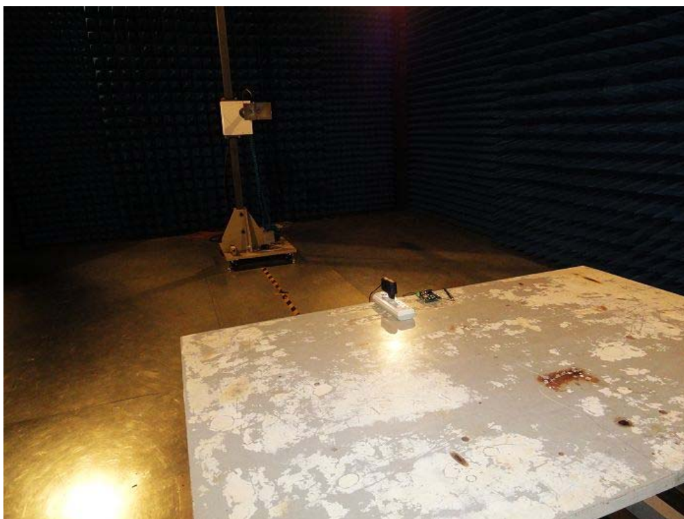
Radiated Emission Test Setup:
