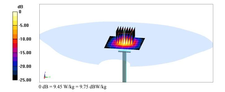
DUT: Dipole 750 MHz; Type: D750V3; Serial: 1054
