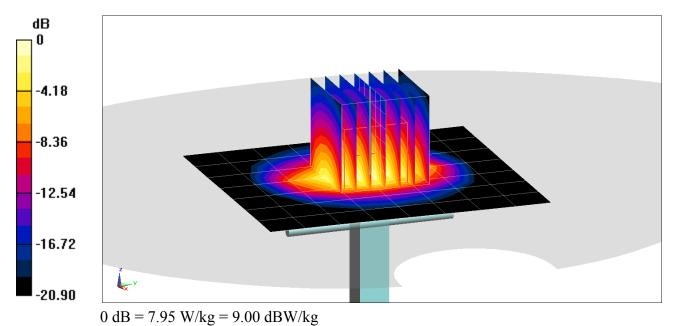
DUT: Dipole 2450 MHz; Type: D2450V2; Serial: 797
