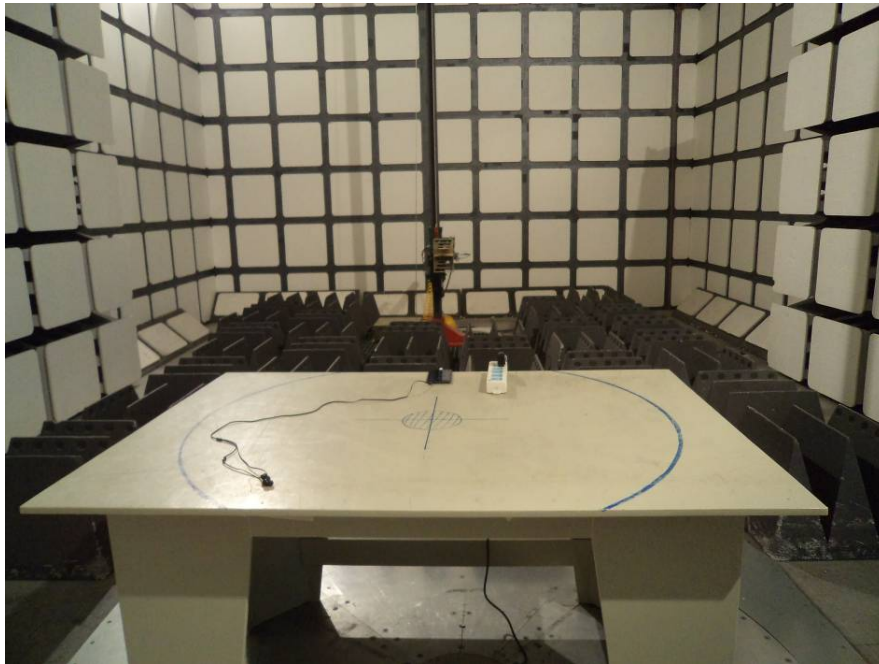
Radiated Emissions Front View (Above 1GHz)
