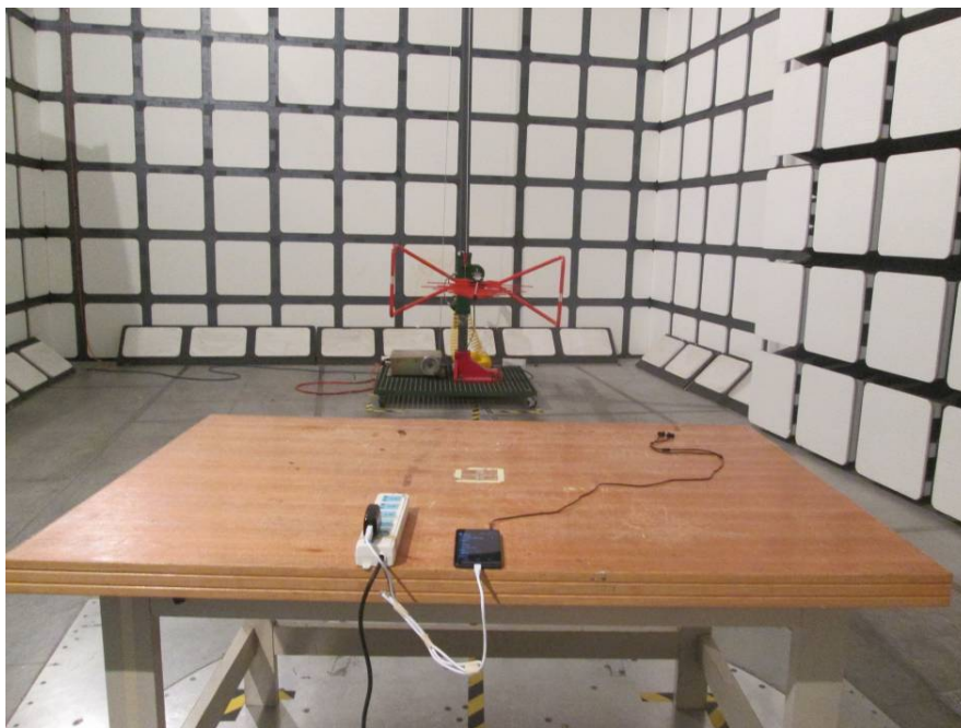
Radiated Emissions Rear View (Below 1GHz)
