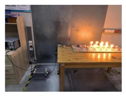
Radiated Emissions From 30MHz-1000MHz
